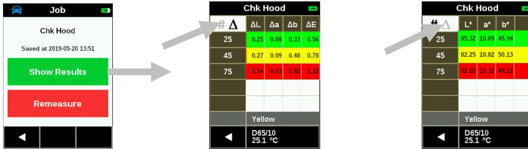
Data fields in tolerance appear green and red for out of tolerance. Data fields can also appear yellow for a close to limit pass.
