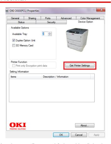
In order to specify system defaults and installed options, administrators select the Printers and Faxes folder from the Microsoft Windows' Start menu, and then select one of the Okidata C610dtn drivers. Administrators can select the "Get Printer Settings" option and installed options will be automatically indicated in the print driver.
