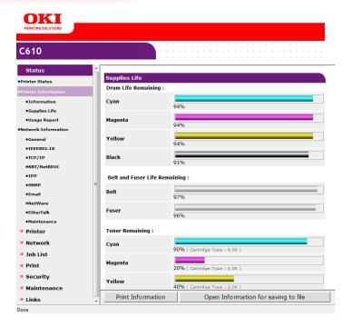
Users can check the status of consumable levels for toner, drum life, transfer belt and fuser units.
