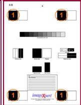
BERTL uses ImageExpert printer test targets for the evaluation of printed image quality. BERTL technicians measure image density and evaluate the device's ability to produce a full range of halftones and various sizes of negative/positive text, dots and lines in each primary printing color (CYMK).
