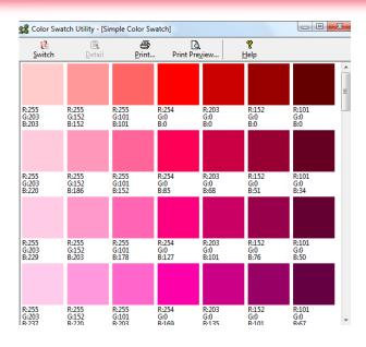
The Color Swatch Utility enables users to print out charts that indicate how specified colors will appear when printed by the device.
