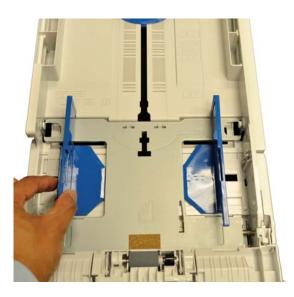
**Above and next page:** In order to adjust all the paper drawers to accommodate different paper sizes, the user squeezes and slides these blue guides into place. BERTL found it easy to adjust the paper drawers.
