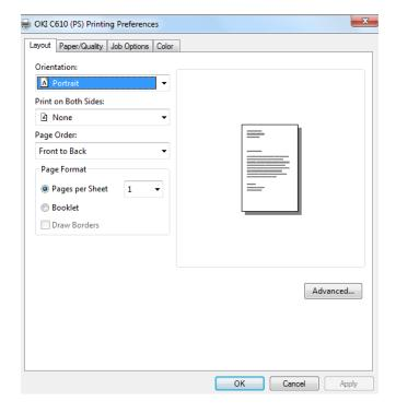
The PostScript driver offers common paper and image quality settings as well as options for storing files to a SD card and secure print (the user is prompted to enter a password which must also be entered at the control panel of the device in order for the job to print).
