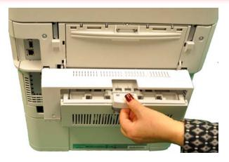
The duplex misfeed-access area is located on the back of the printer. The user simply presses this gray release button and lowers the panel down.
