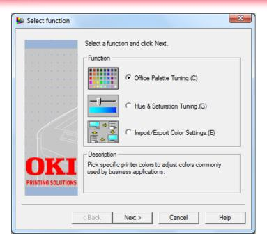
Above and below: The Color Correct utility is designed to help adjust how RGB colors are printed. As well as making it easier for users to adjust colors commonly found in applications such as Microsoft® Word, Excel® and PowerPoint®. This utility also lets users adjust the overall color of a print by controlling the lightness, darkness and contrast of images, and the intensity and lightness of the colors.
