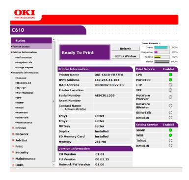
The PrintSuperVision's Printer Status page provides device status, installed paper sizes, and installed options. Additional information includes toner status, print services enabled, and version information.
