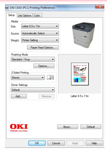
The PCL driver's first tab Setup provides basic options such as paper size, source, weight, finishing mode, duplexing, etc. The image in the lower right indicates the currently selected settings.
