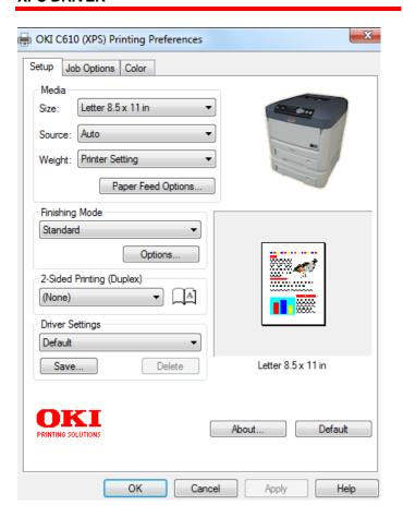
The XPS driver is virtually identical to the PCL5c and PCL6 drivers, providing a bidirectional communication between a user's PC and device eliminating the need for users to manually update the devices components. This driver offers the most common paper and image quality settings.
