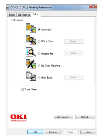
The Color tab provides options that include Automatic, Office Color, Graphic Pro, No Color Matching and Grayscale. These options allow the printer to adjust the colors specified in the document and print them accordingly.
