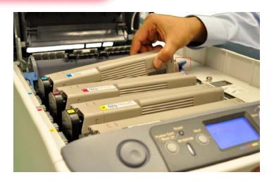
**Above and below:** Once the cover is open, the user can then replace the toner cartridges by turning the blue levers forward and lifting the toner out for replacement.
