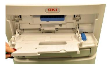
The 100-sheet multi-purpose tray can be adjusted by sliding these levers into place.
