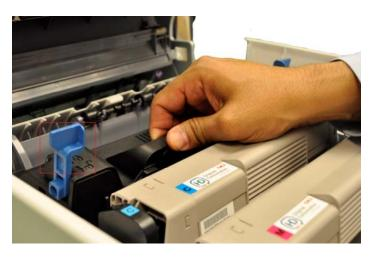
**Above and below:** The printer's fuser unit must periodically be replaced. The user first opens the top cover; the fuser is located toward the back. The user must be careful, as, if the printer has been powered on, the fuser will be hot. The user then unlocks the blue levers and, grasping the fuser by its handle, pulls it out.
