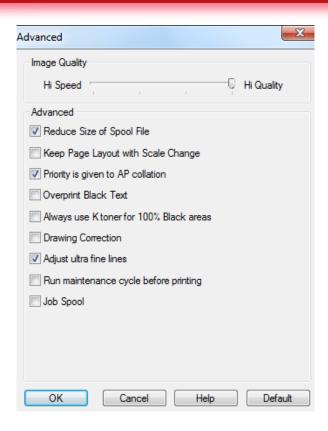
The Job Options' tab provides a link to an Advanced tab that provides options for reducing spool files; overprint black text, adjust ultra fine lines and etc.
